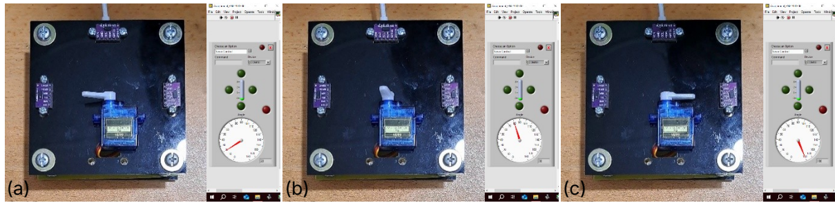
Figure 5: Prototype Servo and LabVIEW response Servo motor controls: (a) 20°, (b) 80°, and (c) 180°
