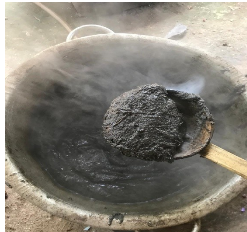
Figure 8: The mixture pastes after heating just before pouring into the mould.
